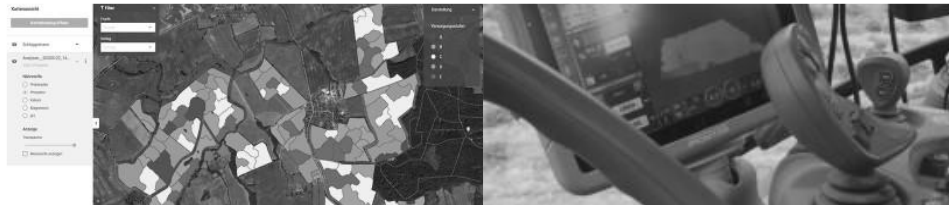
Fig. 1: Left: Predict vegetation levels from satellite images and optimize fertilizer using machine learning. Right: Transfer fertilizer estimations to tractor for precise distribution.
